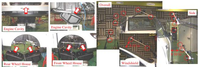
Figure 3: Typical loudspeaker and microphone locations for ideal load testing
