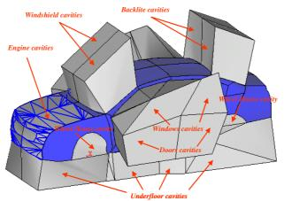
Figure 4: Exterior cavities for which SPL is constrained with measured data
