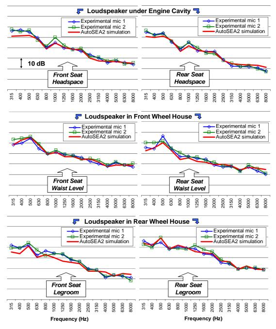
Figure 5: Interior cavities SPL validation results for various load cases
